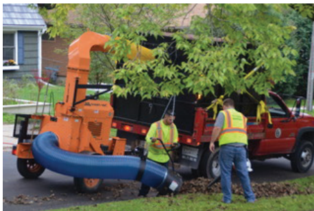
Figure 1. Vacuum assisted equipment used to do weekly leaf pickup in the Wingra study area.
